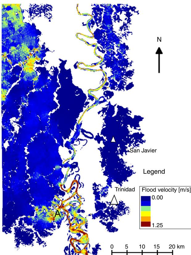
**Fig. 7.** Flow velocity on February 25, 2014 simulated by HEC-RAS.
