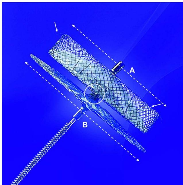
**Figure 1** The Amplatzer™ Cardiac Plug. The Amplatzer™ Cardiac Plug consists of a distal lobe (broken white line A) and a proximal disk (broken white line B) which are connected by a short articulating waist (white circle). The lobe has up to six additional stabilizing wires (white arrows) to assure device retention. The A/B ratio is unique for each device (e.g. for a 20 mm lobe, the A/B ratio is  $20/24=0.833$ , and for a 26 mm lobe, the A/B ratio is  $26/32=0.8125$ ).
