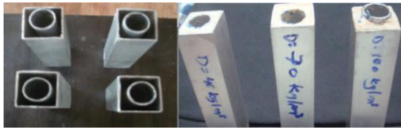
Fig. 11. Experimental specimen of empty and filled concentric tubes [33].
