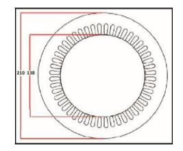
Fig. 2. Schematic of the stator core (dimensions in millimeters).
