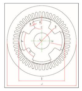
Fig. 5. Rotor quotas in cross-section.
