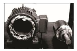
Fig. 1. Three-phase induction motor 10 HP partially disassembled.
