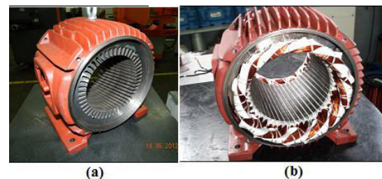
Fig. 12. Assembly stator (a) inserted into the housing, (b) machine coiled.
