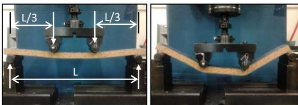
Fig. 1. Third-point loading configuration for four-point bending tests, according to ASTM C 393-00. Test of sandwich specimen with MWCNT-modified adhesive at an early stage (left) and after failure (right) due to core compression.
