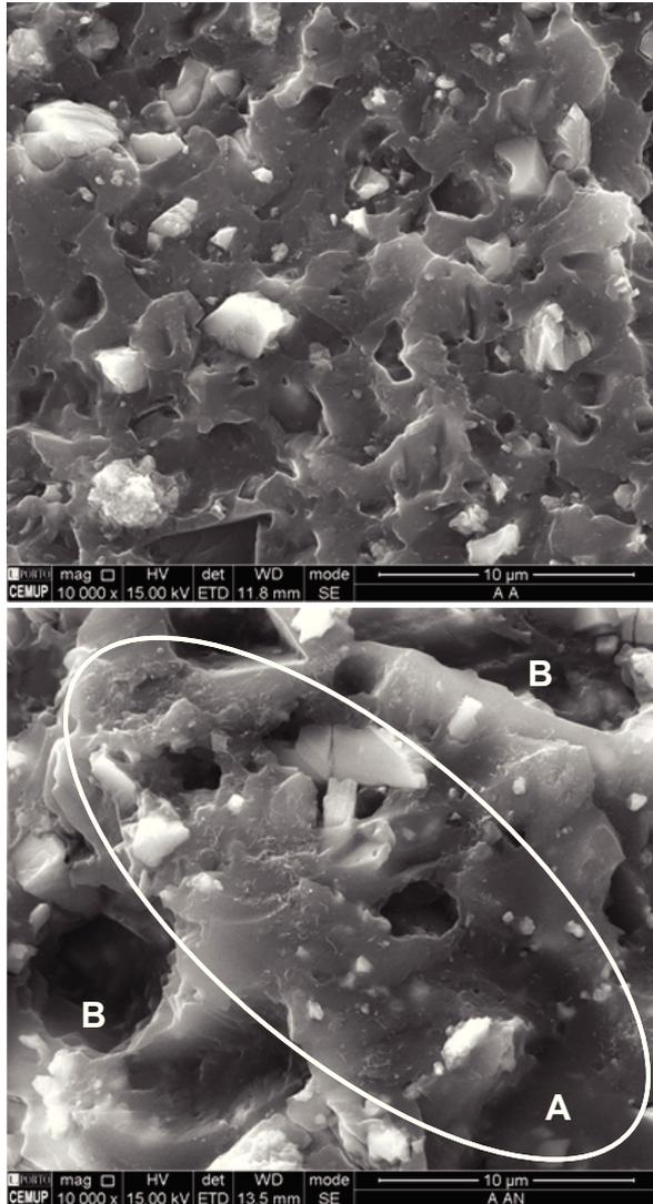
Fig. 2. SEM micrographs obtained at 10000x magnification for both neat (above) and MWCNT-modified (below) adhesives. In the lower picture MWCNT rich (A) and poor (B) areas are identified.
