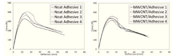
Fig. 4. Load-deflection curves for four-point bending of sandwich structures with (left) neat and (right) MWCNT-modified adhesives.
