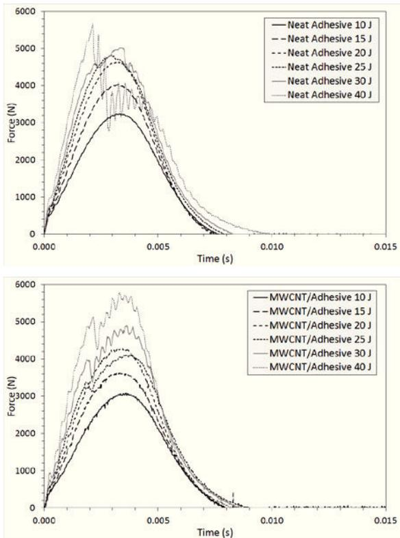
Fig. 5. Force-time plot histories of low velocity impacts for all energy levels, of sandwich specimens with neat (top), and modified (bottom) adhesives.
