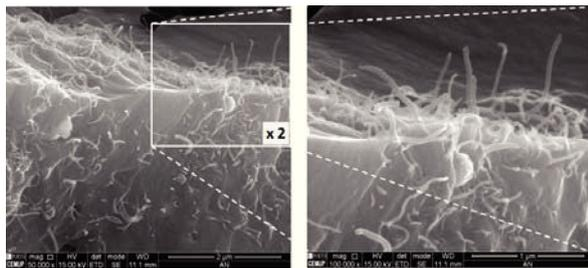
Fig. 3. SEM micrographs obtained at 50000x and 100000x magnification MWCNT-modified adhesive showing CNT rich and poor areas in the foreground and background, respectively.
