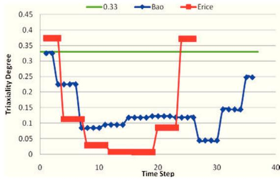
Fig. 24. Stress triaxiality degree development into the two types of specimens.
