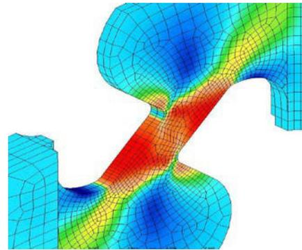
Fig. 14. Detail of the area with stress concentrators when the Bao specimen undergoes shear stress.
