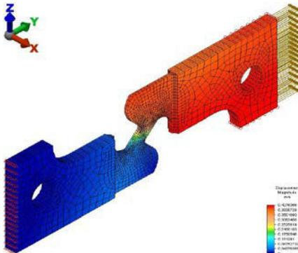
Fig. 13. Displacement magnitude for Bao specimen.
