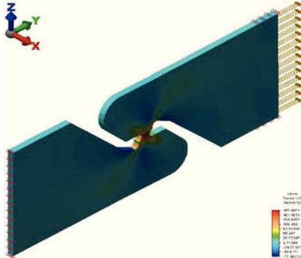
Fig. 6. Shear stress for Erice specimen.
