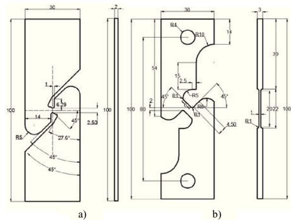
Fig. 1. Geometric shape and dimensions.
