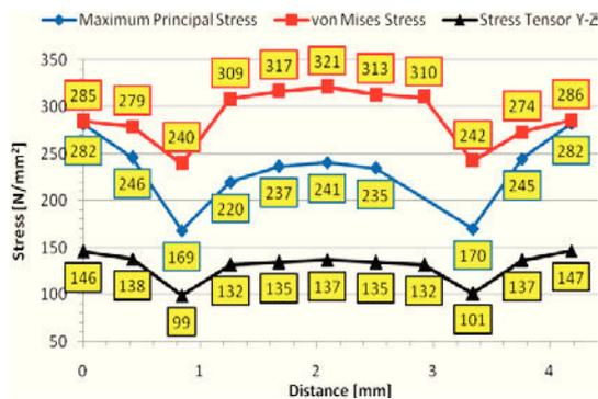
Fig. 17. Stress diagram for Bao specimen.
