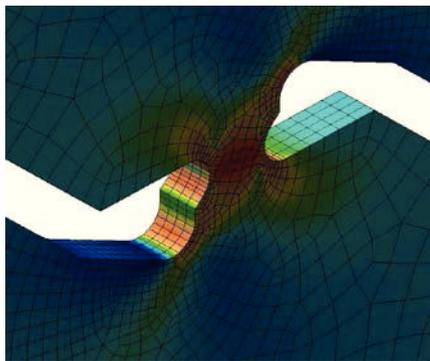
Fig. 7. Detail of the area with stress concentrators when the Erice specimen undergoes shear stress.
