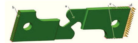
Fig. 9. Loadings and boundary conditions for Bao specimen (a - specimen with stress concentrators, b - embedding, c - guidelines, d - uniform loading).
