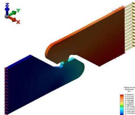
Fig. 5. Displacement magnitude for Erice specimen.
