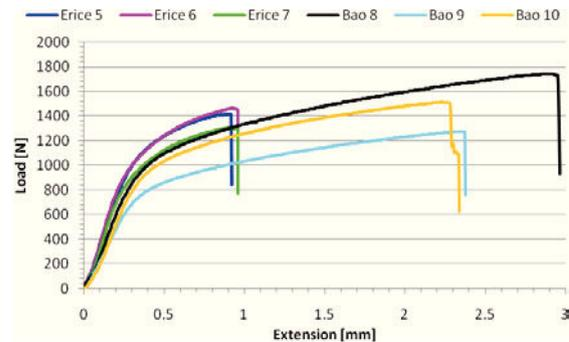
Fig. 23. Load-elongation diagram (specimens 5 to 10).
