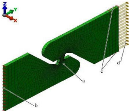
Fig. 2. Loadings and boundary conditions for Erice specimen (a - specimen with stress concentrators, b - embedding, c - guidelines, d - uniform loading).
