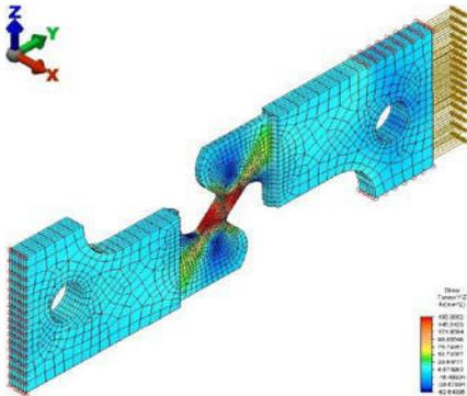
Fig. 12. Shear stress for Bao specimen.
