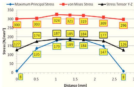
Fig. 16. Stress diagram for Erice specimen.
