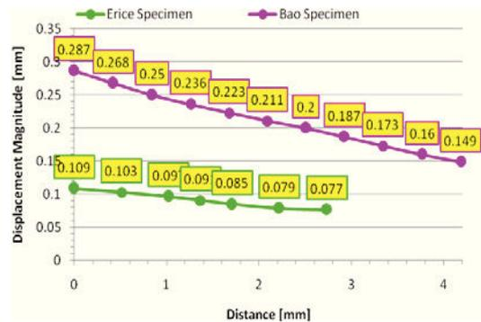
Fig. 18. Displacement magnitude diagram for both specimens.
