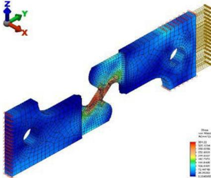
Fig. 11. Von Mises stress for Bao specimen.
