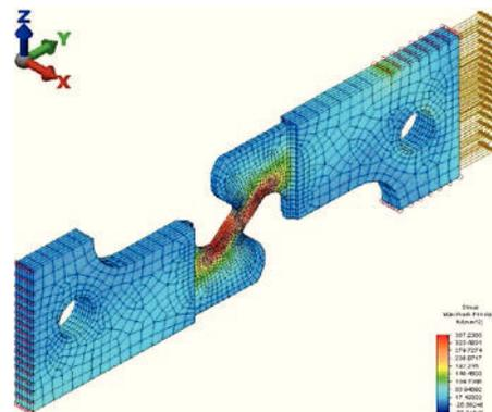
Fig. 10. Maximum principal stress for Bao specimen.
