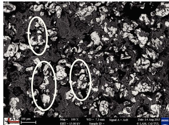
Fig. 11. SEM image of fillers arrangement in elastomeric matrix composite.
