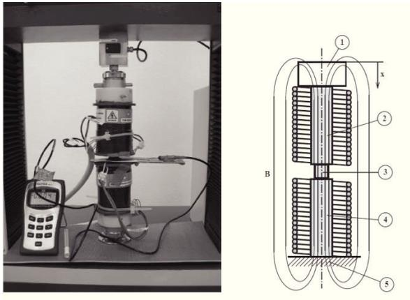
Fig. 8. Photographic and schematic diagram of compression test in closed magnetic domain. (1 - Dynamometr TIRA, 2 and 4 – ferromagnet, 3 - MRE sample, 5 - frame of TIRA).
