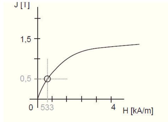
Fig. 5. Characteristic of core (steel) intensity versus magnetic induction.
