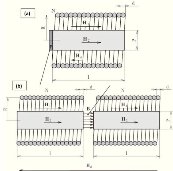
Fig. 4. (a) Schematic diagram of solenoid core. (b) Coupled magnetic core domain.
