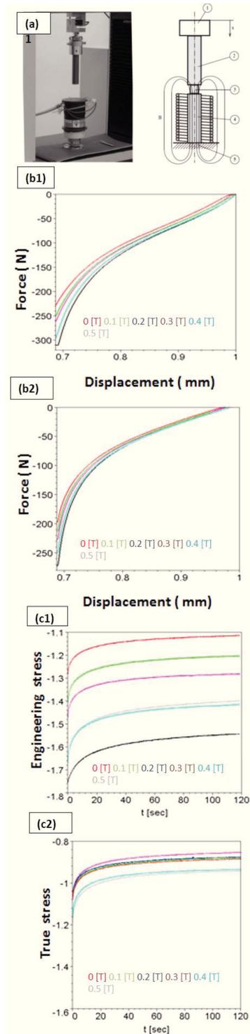
Fig. 7. (a) Photographic and schematic configuration of compression test. (1 - Dynamometer TIRA, 2 - Aluminum metal, 3 - MSE elastomer, 4 - magnetic domain, 5 - frame of TIRA). (b1) Force versus displacement for compression and (b2) relaxation stage at various magnetic intensity. (c1) Engineering stress as the function of time at various magnetic intensity. (c2) True stress as the function of time at various magnetic intensity.
