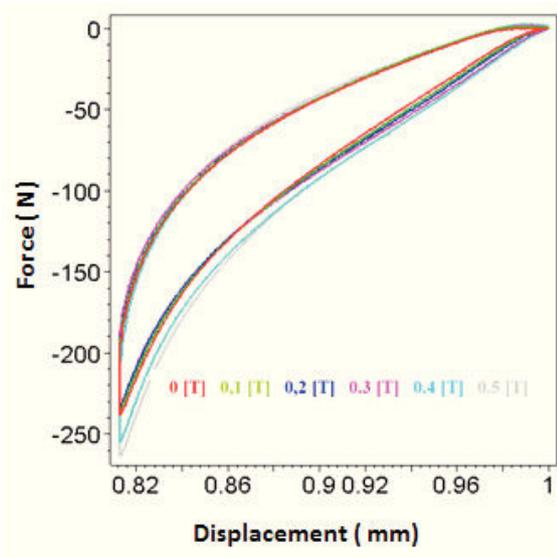
Fig. 9. Hysteresis curve in compression test for MRE samples.
