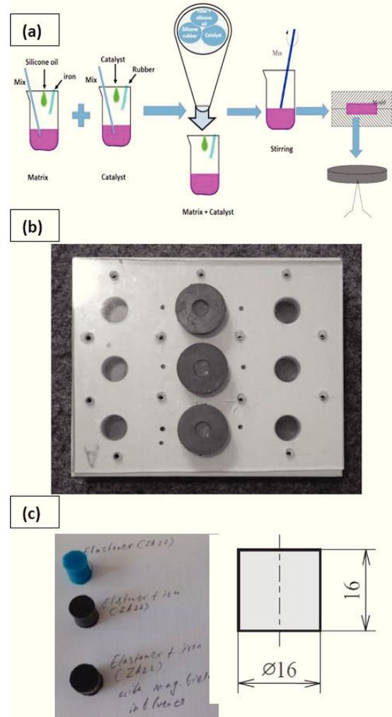
Fig. 3. (a) Schematic diagram of MREs composite formation. (b) Fabrication of sample and curing under magnetic field. (c) Photographic image and sample dimension of MRE composite.
