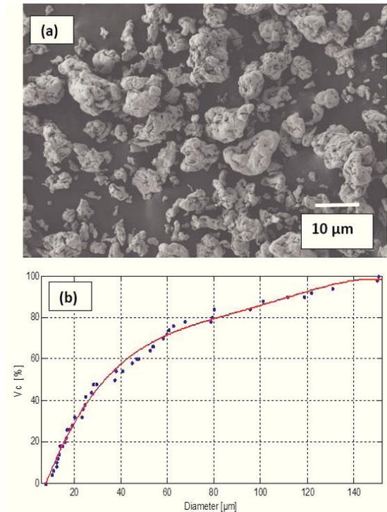
Fig. 2. (a) Scanning electron microscope image of iron filler. (b) Dependence of volume fraction (cumulative frequency) as the function of particle size for iron particles.
