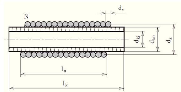
Fig. 6. Schematic diagram of measuring coil.
