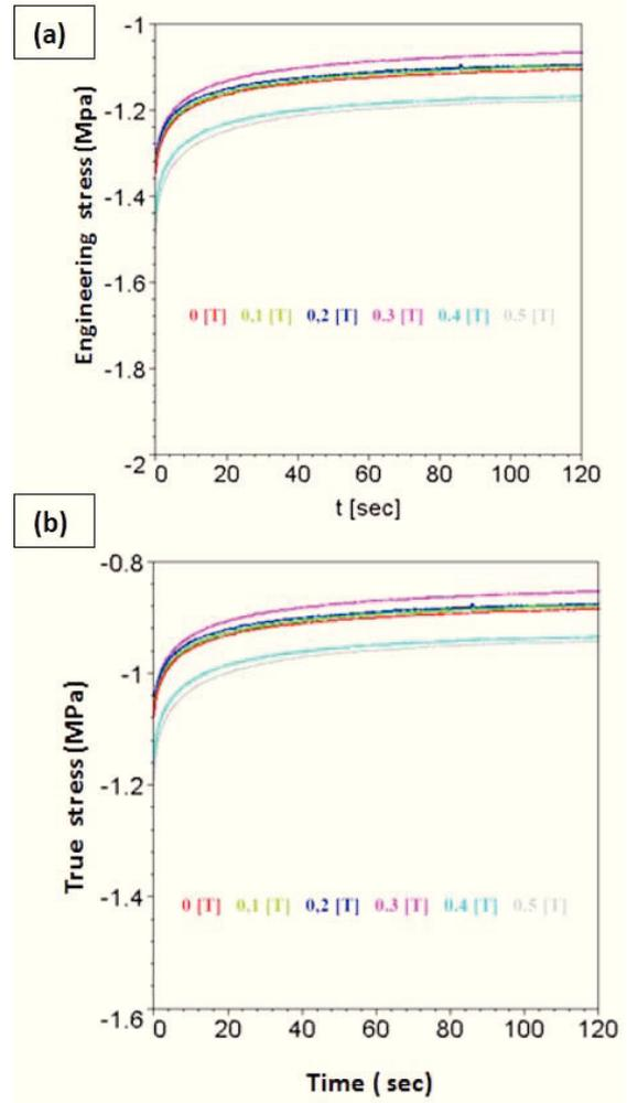
Fig. 10. (a) Engineering stress as the function of time at various intensity. (b) True stress of the MRE composite as the function of time at various intensity.
