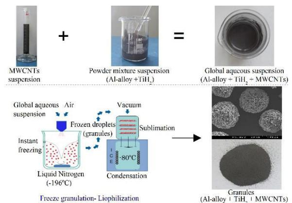
Fig. 1. New colloidal processing step add to the powder metallurgy method. Highly-spherical granules prepared by FG-Lyophilisation.
