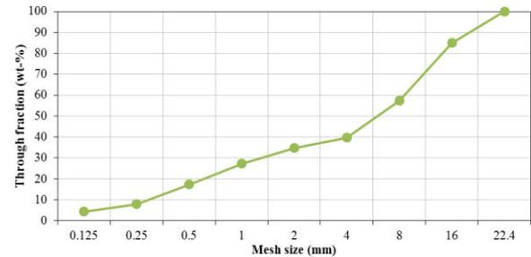
Fig. 1. Particle size distribution of the aggregates used in the tests.
