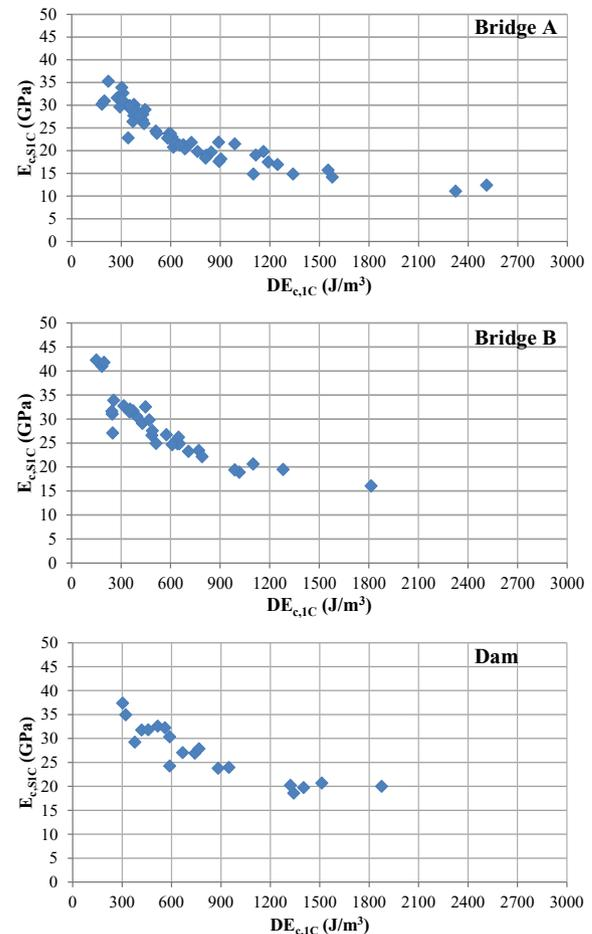
Fig. 2. Representation of the elasticity modulus (obtained from the slope of the first load/unload cycle) versus the energy dissipated during the first load/unload cycle obtained for cores extracted from two concrete bridges and one concrete dam.
