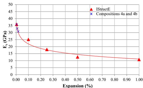
Fig. 3. Representation of the elasticity modulus (obtained from the slope of the first load/unload cycle) versus the expansion obtained for the reference concrete and for concrete compositions 4a and 4b. Overlaid in the same graphic is the variation of the elasticity modulus with the expansion due to ASR according to IStructE [11] for expansion values higher than 0.10 %.
