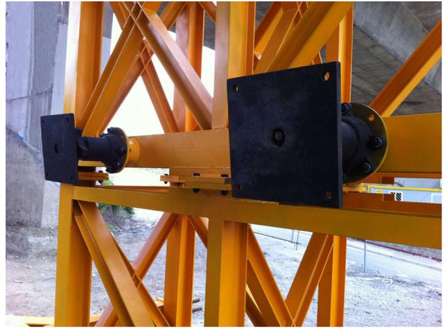
Figure 22. Bumpers fitted with spherical hinges and regulation screw spindle.
