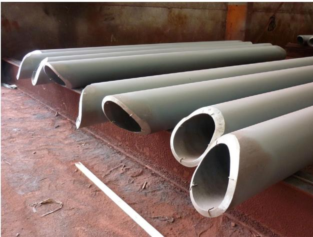
Figure 10. Cuts and preparation of the edges of the tubes forming the diagonals of the latticework.
