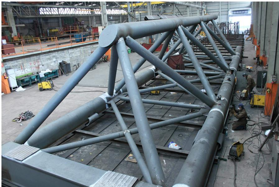
Figure 23. Mounting the deck latticework at the workshop.
