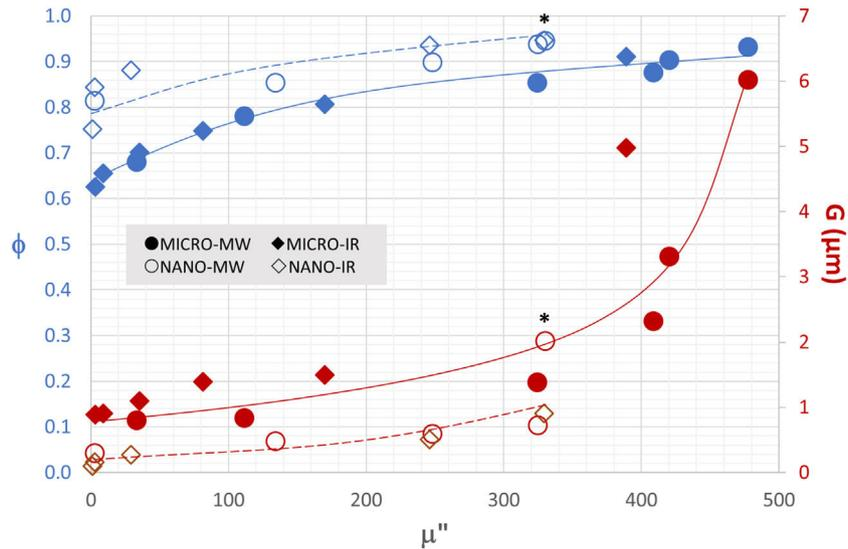
Fig. 7 – Imaginary part ( $\mu''$ ) of the complex magnetic permeability dependence of relative density (blue) and average grain size (red) for the two studied granulometries (MICRO and NANO) sintered with both infrared radiation (IR) and microwaves (MW).
