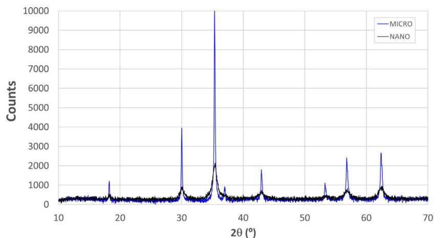
**Fig. 2 – X-ray diffraction patterns of the MICRO and NANO starting powders corresponding to the crystal structure of NiZn(Fe<sub>2</sub>O<sub>4</sub>).**
