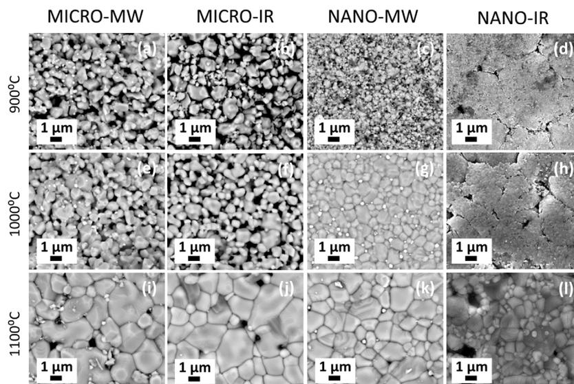
**Fig. 4** – Scanning electron microscopy (SEM) images for the sintered MICRO-MW samples at 900 °C (a), 1000 °C (e) and 1100 °C (i); the MICRO-IR samples at 900 °C (b), 1000 °C (f) and 1100 °C (j); the NANO-MW samples at 900 °C (c), 1000 °C (g) and 1100 °C (k); and the NANO-IR samples at 900 °C (d), 1000 °C (h) and 1100 °C (l).
