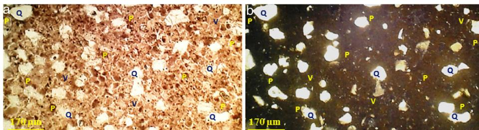
**Fig. 6 – Micrography of the fired refractory specimen M6 mixed with 25% of Rec-Al at 1500 °C. (a) Natural microscopy light (AL). (b) Polarized microscopy light (APL). P: Porosity, Q: Quartz, V: Vitreous phase.**
