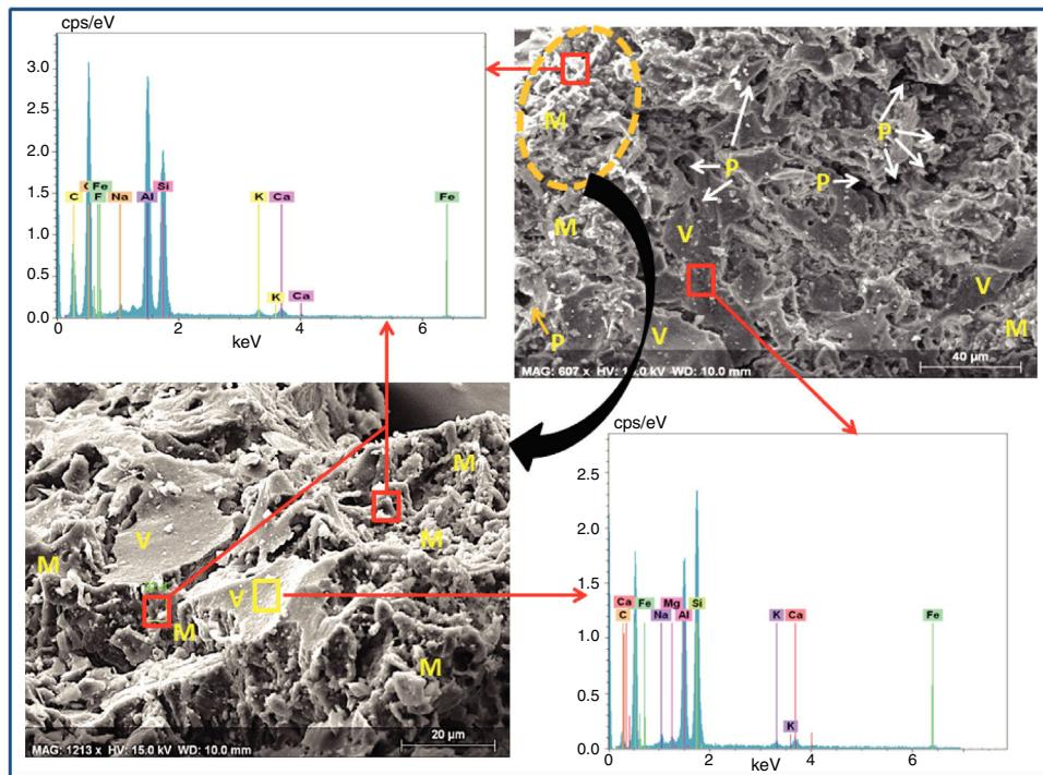
**Fig. 7 – SEM images of the fired specimen of sample M6 mixed with 25% of Rec-Al at 1500 °C a and associated EDS spectra. P: Porosity, V: Vitreous phase, M: Mullite.**
