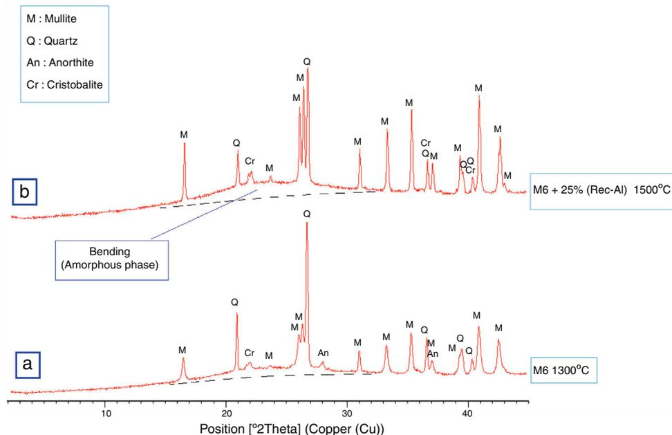
Fig. 8 – XRD spectra of sample M6 fired at 1300 °C (a), and sample M6 mixed with 25% of Rec-Al fired at 1500 °C (b).
