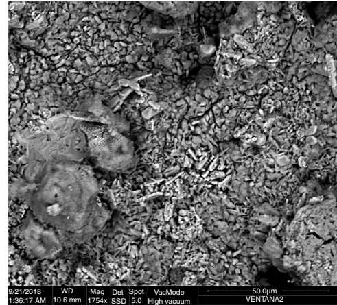
Fig. 8 – BSE image of the material collected from the hot face of the refractory brick samples located in the gas area of the lining of the SAF. An analysis of the hole image was carried out and the result is shown in Table 1 (analyzed point W, window).
