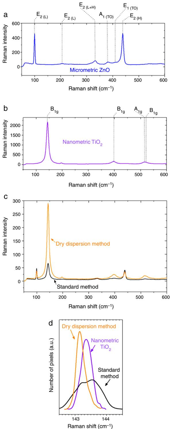
**Fig. 5 – Raman spectra of (a) micrometric ZnO, (b) anatase nanometric TiO<sub>2</sub> raw material, and (c) composites by dry dispersion method and mixed oxides by the standard method compared with the anatase nanometric TiO<sub>2</sub> raw material. (d) Statistic distribution of the Raman shift for B<sub>1g</sub> Raman mode for both dispersion methods in comparison with the raw material.**
