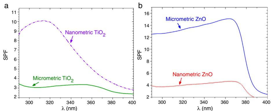
Fig. 3 – SPF curves of COLIPA sunscreen incorporating inorganic UV filter: nanometric (dashed lines) and micrometric (solid lines) of (a) TiO<sub>2</sub> and (b) ZnO particles.
