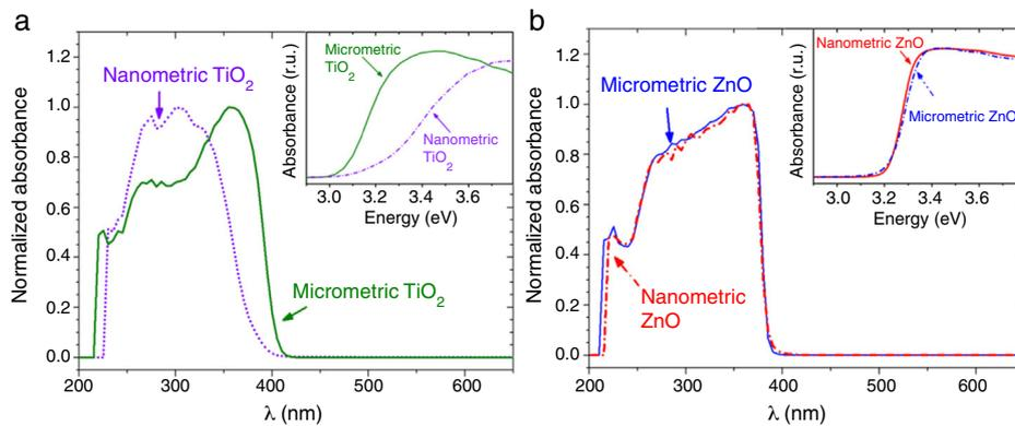
Fig. 2 – UV-vis absorption spectra of the nanometric (dashed lines) and micrometric (solid lines) UV filters: (a) TiO<sub>2</sub> and (b) ZnO. The insets represent their corresponding plots of transformed Kubelka–Munk function versus the energy of light.
