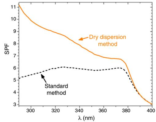
**Fig. 6 – SPF curves of sunscreens with micro-nano composite filters. Straight line represents the SPF curve of new micro-nano composite obtained by nanodispersion method and dash line by a standard method.**
