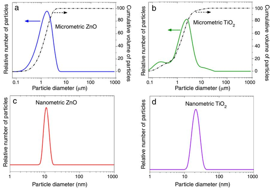
Fig. 1 – Particle size distribution of (a) micrometric ZnO, (b) micrometric TiO<sub>2</sub>, (c) nanometric ZnO, and (d) nanometric TiO<sub>2</sub>.
