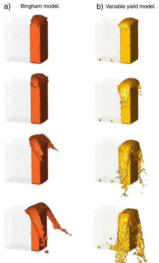
Fig. 6. 3D pushed slope. Difference between the Bingham and the variable viscosity models in the squeezing phase.
