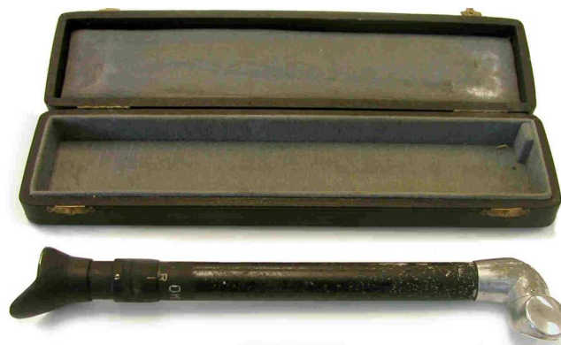
Figura 1 Fluoroscopio intraoral (cortesía de Paul Frame de Oak Ridge Associated Universities).
