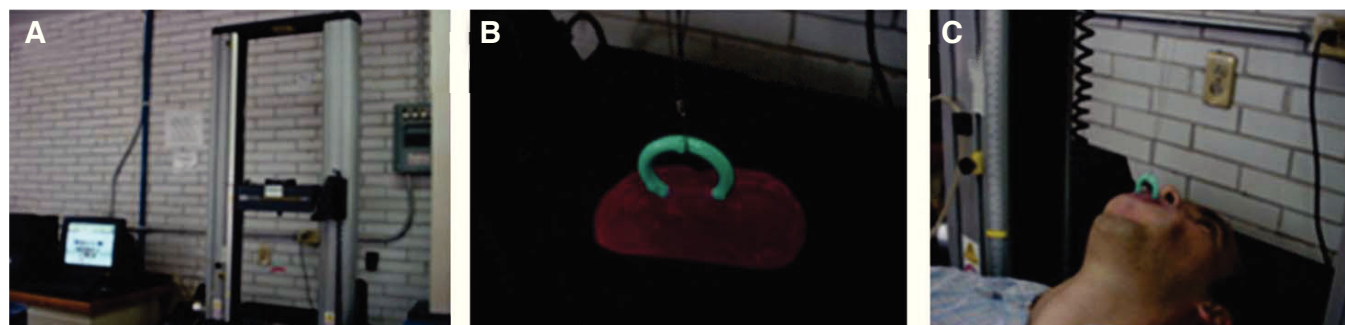
Figure 4. In vivo stress test. A) Universal testing machine. B) Buccal shield. C) Stress test.
