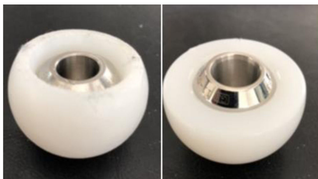
Figure 2 28mm head and polyethylene of the two systems. Quattro™ and Dualis™, respectively.
