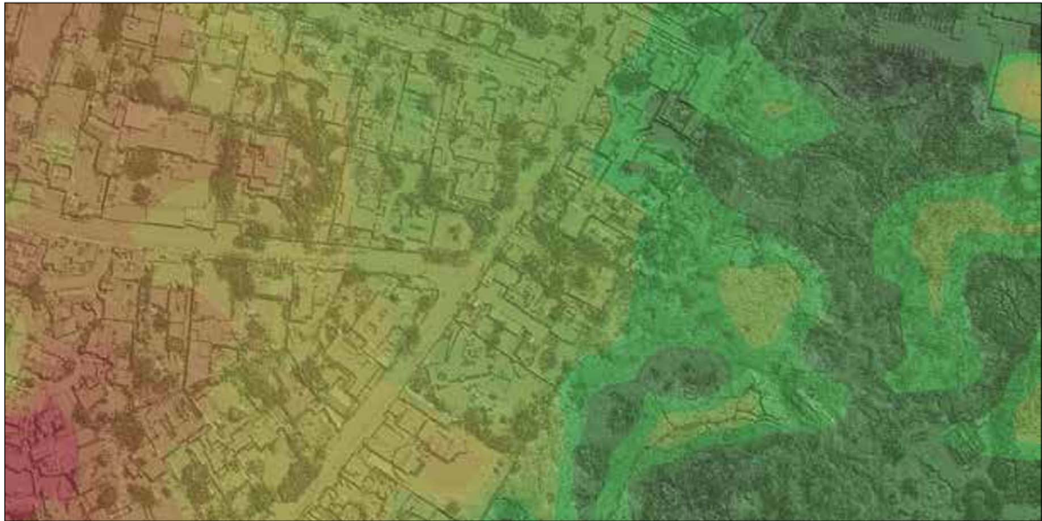
Figure 1. Digital Surface Model (DSM) reported onto the Digital Terrain Model (DTM) (bare earth surface using a colored hypsometric scale [green to red]) generated from the point cloud.
