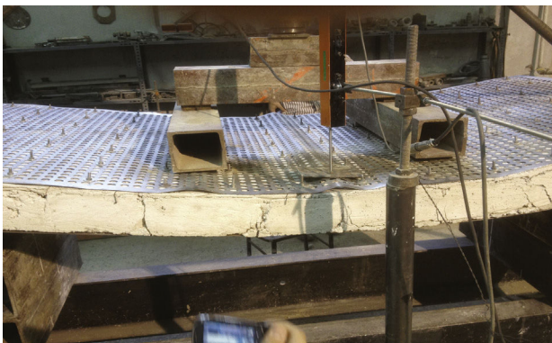
Figure 5. Buckling of the compression plate
