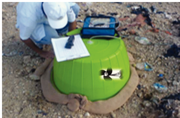
Figure 2. Static chamber technique applied in Merida landfill
