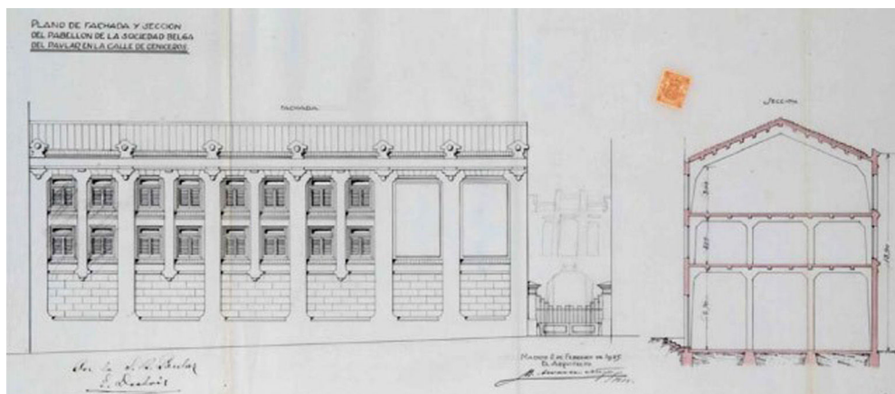
Figure 14. Original drawings by architect Manuel Álvarez Naya (1925). All structure elements—columns, beams, joists and slabs—are visible in the section.
