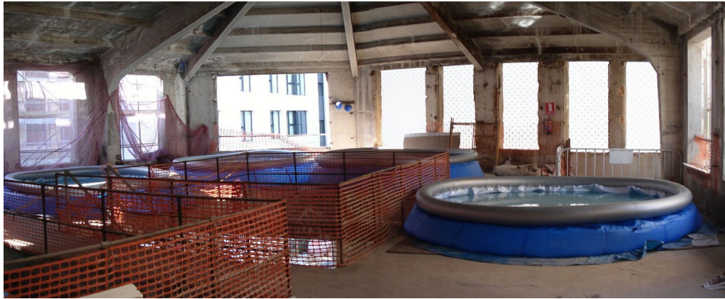
Figure 17. Water containers used for the load test.
