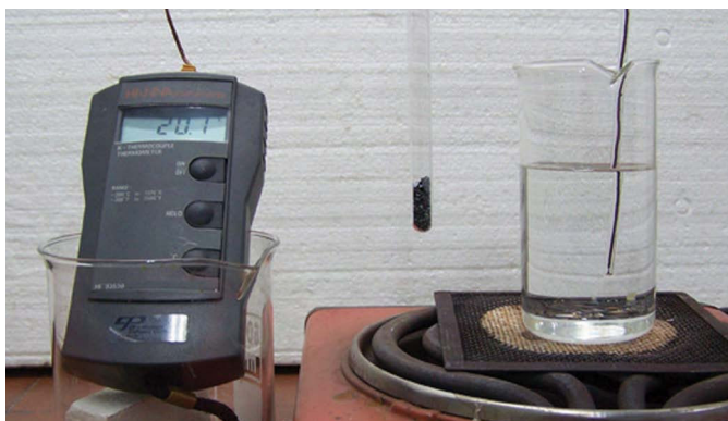
Figure 2. Melting of iodine, the experimental setup: digital thermometer (left), test-tube with iodine (middle) and the glycerol bath with the thermocouple (right).
