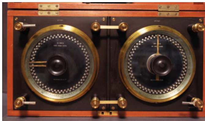
Figure 3. Left: Photograph of a historic induction apparatus of about 1874 taking the function of (6) of Fig. 2. Right: photograph of a resistor box taking the function of (1) of Fig. 2. The age of this box is unknown. It could however correspond to a commercial model available at Alfred Werner's time. Both instruments were located in the archives of the Physics Institute of the University of Zurich. In principle these instruments could have been used by Alfred Werner and his group, whether they were used by them is not reported.
