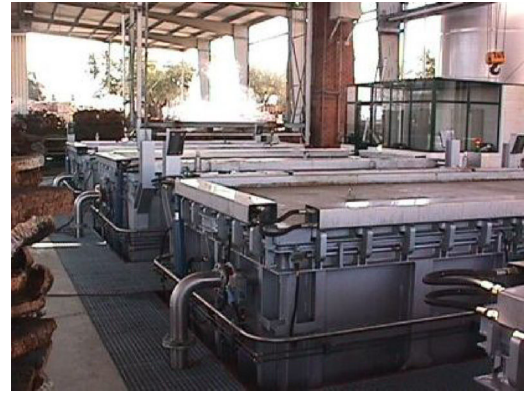
Fig. 2. Cork boiling steel tanks.
