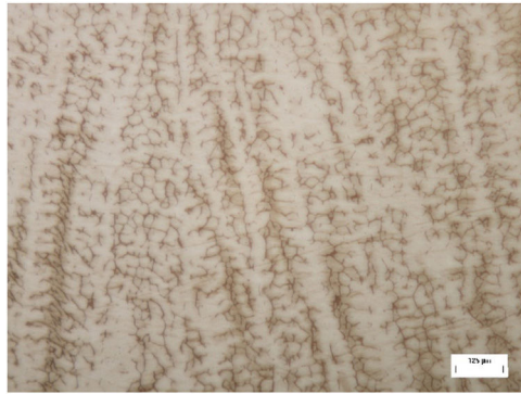
Fig. 16. AISI 316L MZ, heat input of 0.5 kJ/mm. Image obtained with increase of 200× in optical microscope, chemical attack performed with reagent Beraha.
