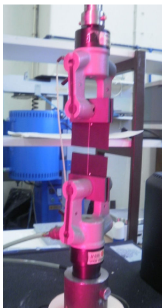
Fig. 6. Specimen clamped with pneumatic grips and illuminated by the video extensometer, during a tensile test, where the yarn deformation is already meaningful.
