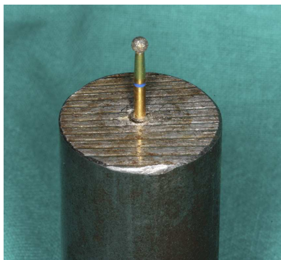
Fig. 5 – The spherical bur after being polished with a diamonded disc and included into a steel cylinder with cyanoacrylate glue (Henkel Co., Germany).
