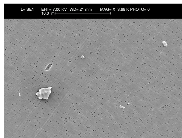
Figure 3 Smaller polyethylene particles are shown in the scanning electron microscope 20,000× images. The quality of the sample can also be seen, showing the correct digestion and filtration of the same, as the image is clear and the filter pores are clearly visible.
