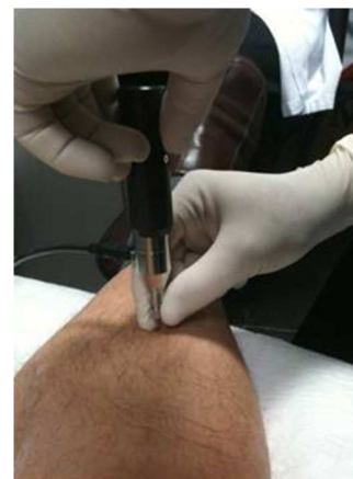
Figure 2 Microindentation technique applied at the level of the tibial diaphysis.
