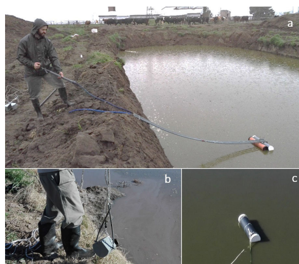
Figure 1 Device used for sampling. (a) Water extraction pump system with manual pump; (b) sediment collection dredge; and (c) surface buoy for Moore swabs.
