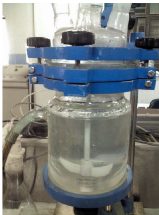
Figure 1 Glass reactor with a mechanic stirrer operating.
