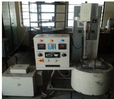
Fig. 1. Compo casting setup.
