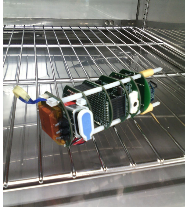
Fig. 4. Assembled structure, ready for starting a vacuum thermal cycle.
