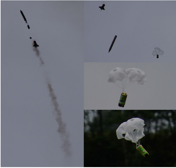
Fig. 12. Separation from the rocket and successful deployment of the parachutes.
