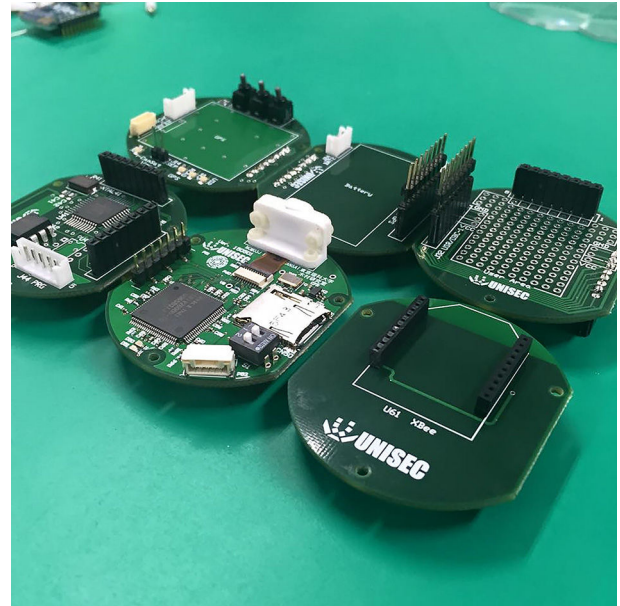
Fig. 1. The six PCB (one for each subsystem), with some soldered electronic components.
