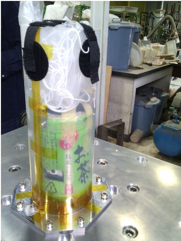
Fig. 6. Full system mounted in the setup for the vibration test.
