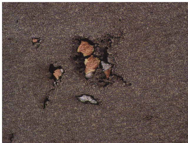
Fig. 5. Clustering of particulates, Al–15% Cu composite, 100 ×.
