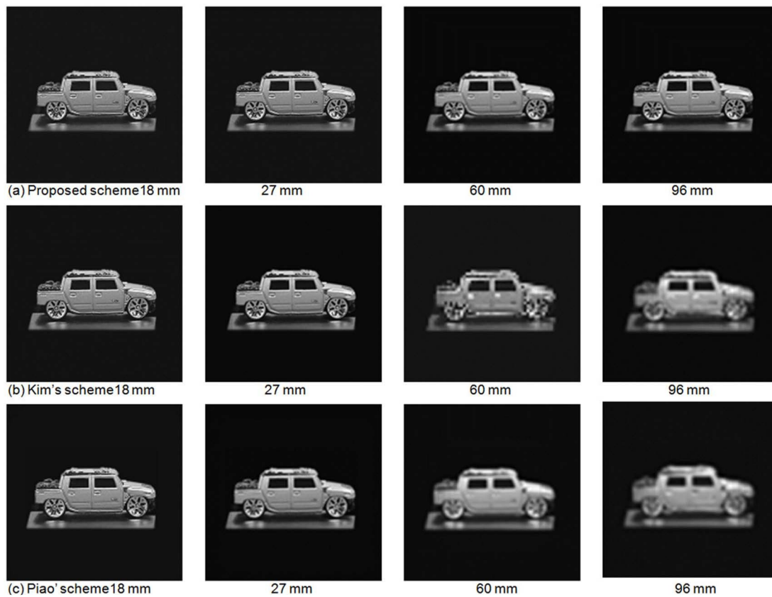
Figure 7. Reconstructed plane images according to the different pickup distances z : (a) the proposed scheme, (b) the Kim et al. scheme, (c) the Piao et al. scheme.
