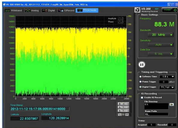
Figure 3. The proposed interface of the TDOA-based monitoring system by selecting the sampling time, filter, bandwidth etc.
