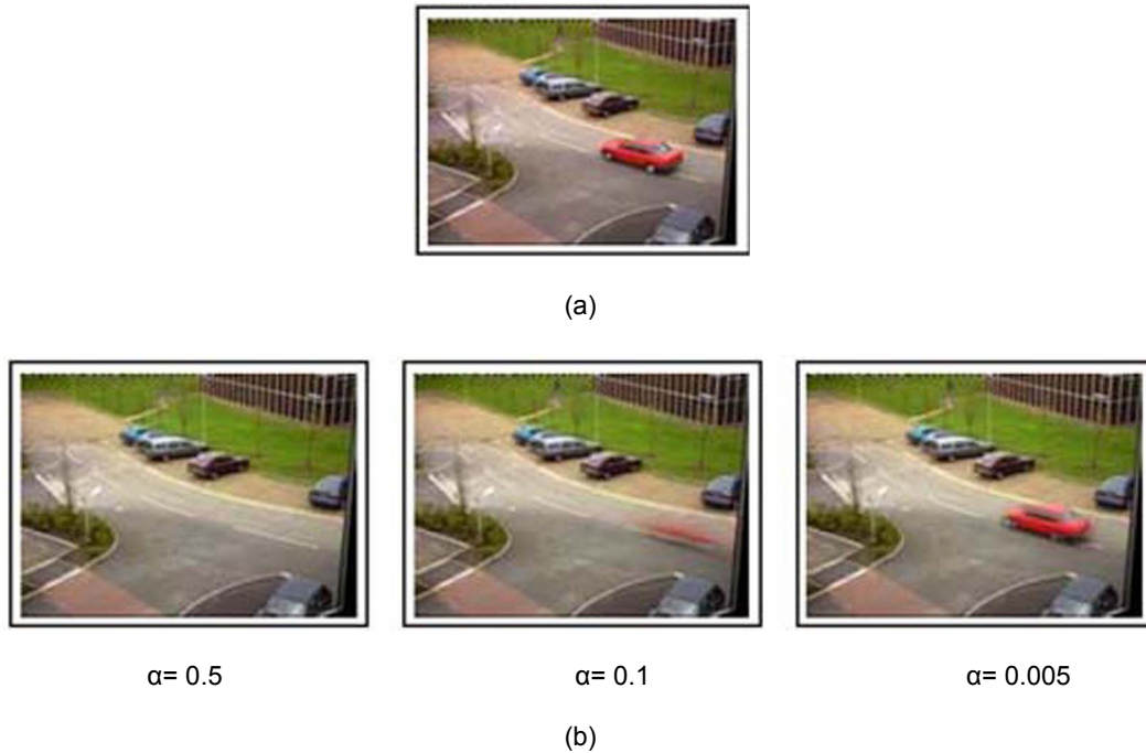
Figure 3. Learning rate speeds at which objects are absorbed by the background model. (a) Original video sequence and (b) visual effect.
