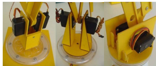
Figure 6. Examples of motor base-rotating bearing table assemblies.
