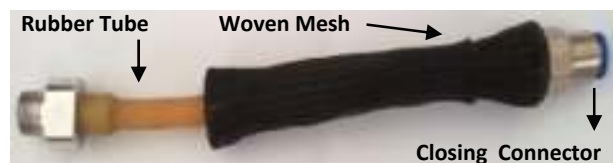
Figure 1. Structure of a pneumatic artificial muscle actuator.
