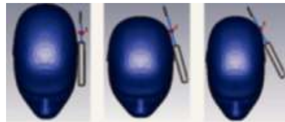
Figure 3. Different position used for SAR measurement: a) Cheek, b) Tilt 150, and c) Tilt 300.
