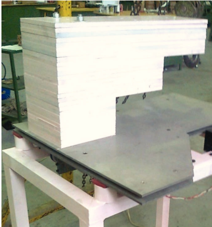
Figure 9. Steel plates simulating mammography equipment weight (250 kg)
