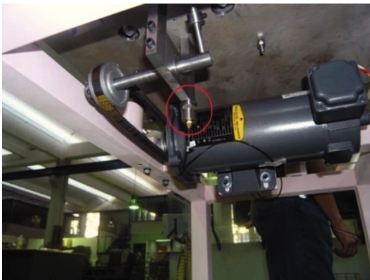
A) Accelerometer below the base of the anti-vibration support system
