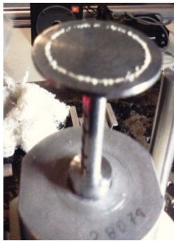
Figure 5. Disk vibrating in a mode with a nodal ring, the sand particles aggregate in the ring where the amplitude of vibration is nearly zero
