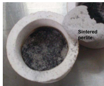
Figure 7. Picture of the sintered perlite taken from the crucible of the arrangement of figure 5 left
