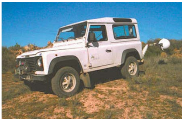
Figure 7. VLF-EM method: equipment adapted to a vehicle (Castelejo mining site).
