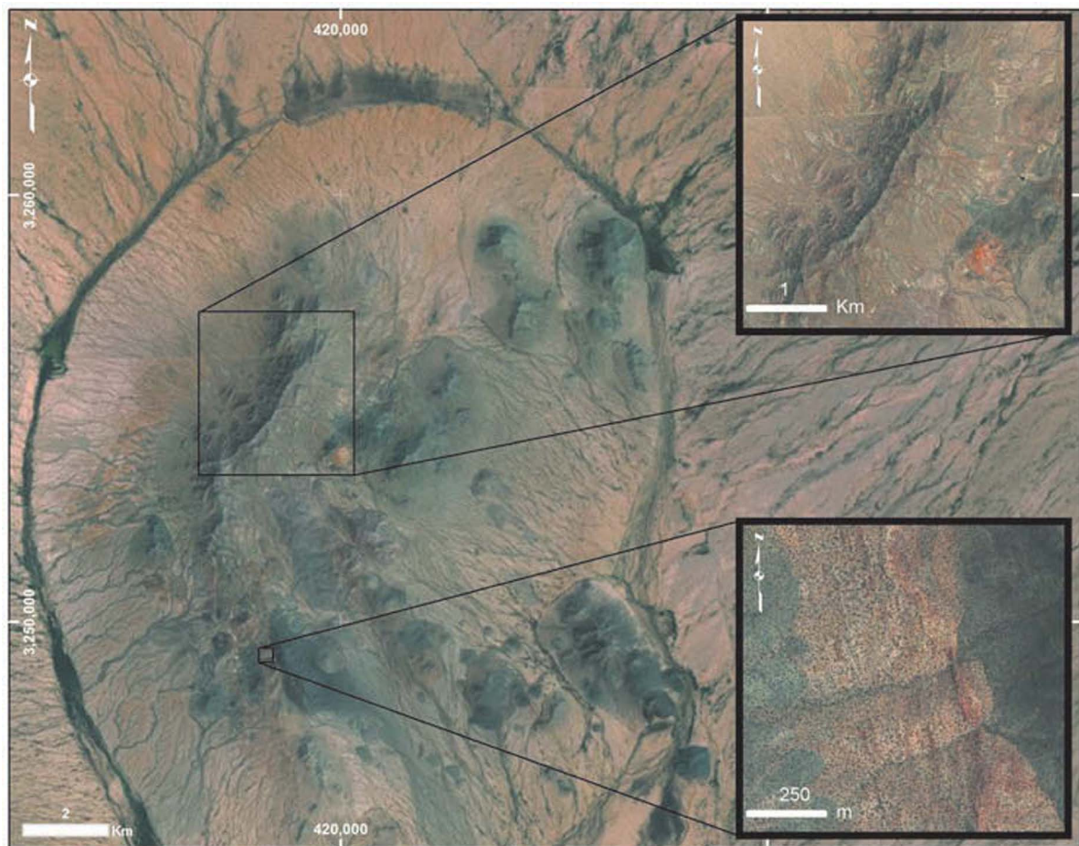
Figure 5. Shows the RNSS and the system of fractures filled of rhyolitic composition dikes. Two detailed images of the dikes in the northern and southern portion are presented. Images taken of Google Earth.
