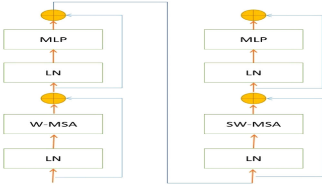
Fig. 3. The constituent modules that constitute the Swin Transformer model. Layer normalization, commonly abbreviated as LN, refers to a technique used in the field of machine learning and neural networks. The abbreviations W-MSA and SW-MSA are used to represent the multi-head self-attention modules with conventional and shifted apertures, respectively.
