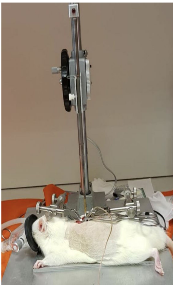
Fig. 2. Spinal impact using the NYU Impactor.
