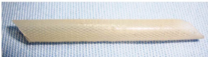
Figure 1 - PDMS prosthesis with a tubular wall of 0.4 mm and an internal diameter of 4 mm.
