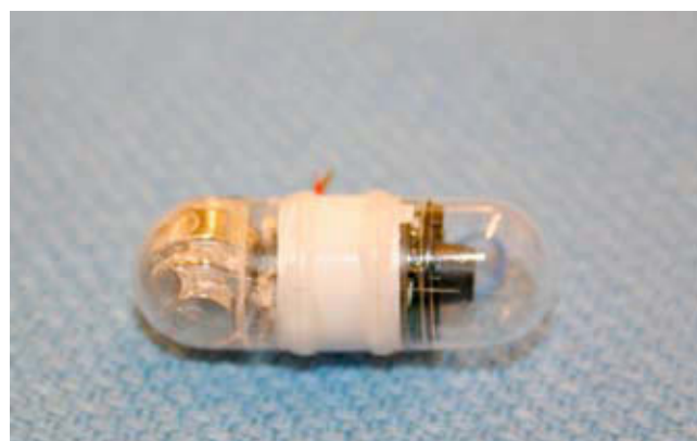
Figure 17 – Wireless Capsule Endoscope (WCE). On the right hand side, the optical system, and on the left the magnetic guidance system. From 35 .
